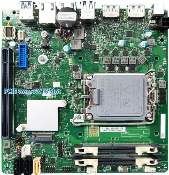
Simply find the appropriate slot for your add-in card and insert the card firmly. Do not force any add-in cards into any slots if they do not seat in place. It is better to try another slot or return the faulty card rather than damaging both the motherboard and the add-in card.
